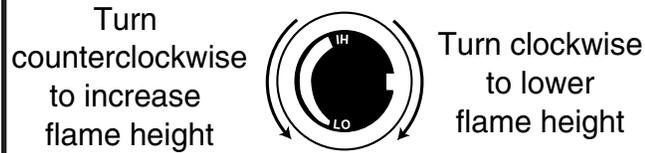
Fig. 15 Flame adjustment knob for SIT820 valve.
